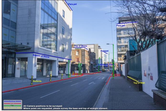
Fig.7: Fixed reference points marked for surveyour.
